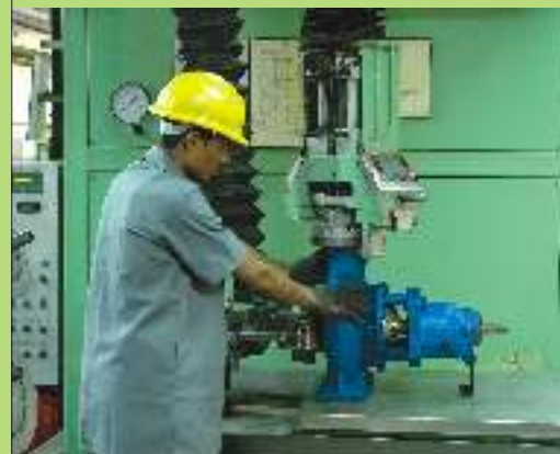
Hydrostatic test of casing
